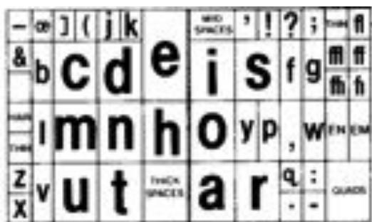
One of the cases in which printers (*Buchdrucker*) kept their letters (metal type). The arrangement (*Anordnung*) of the letters is based on frequency (*Häufigkeit*) of use rather than alphabetical order. The most used letter is e .
