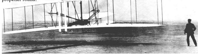
By 1903 the Wright brothers had built *The Flyer*. It was a biplane (with two sets of wings) and the pilot lay flat (flach) across the lower (unterer) wing. A series of bicycle chains (Ketten) and gears (Getriebe) connected the engine to two propellers which rotated at about 450 times a minute. On 17 December 1903, at Kitty Hawk in North Carolina, Orville Wright made a 12-second flight over a distance of 35 m. This was the first aeroplane flight in history.
